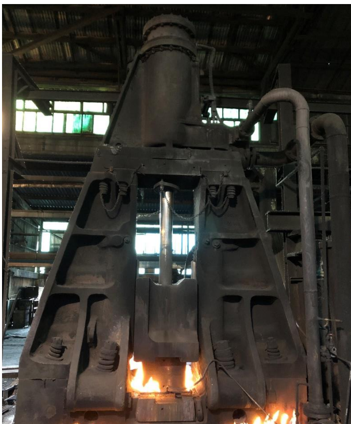
16,000# Chambersburg Power Forge Hammer
