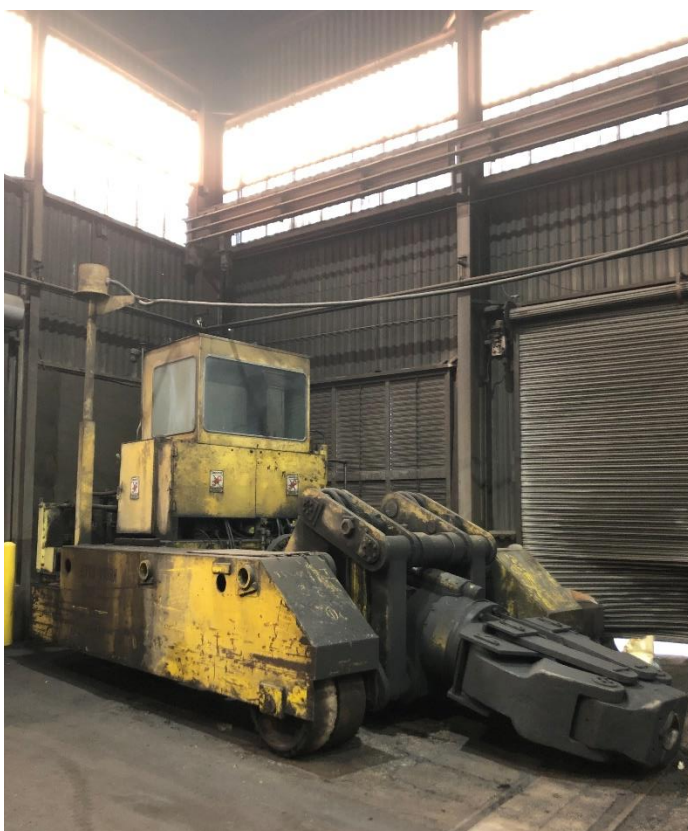
DEC Equipment Corp. 36,000 LB Manipulator
