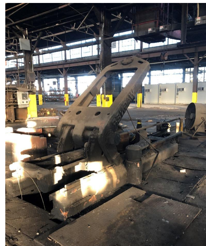
Wagner Ring Roller, 80 Ton Max Roll Pressure
