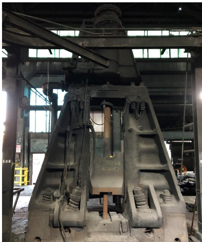
6,000# Chambersburg Power Forge Hammer
