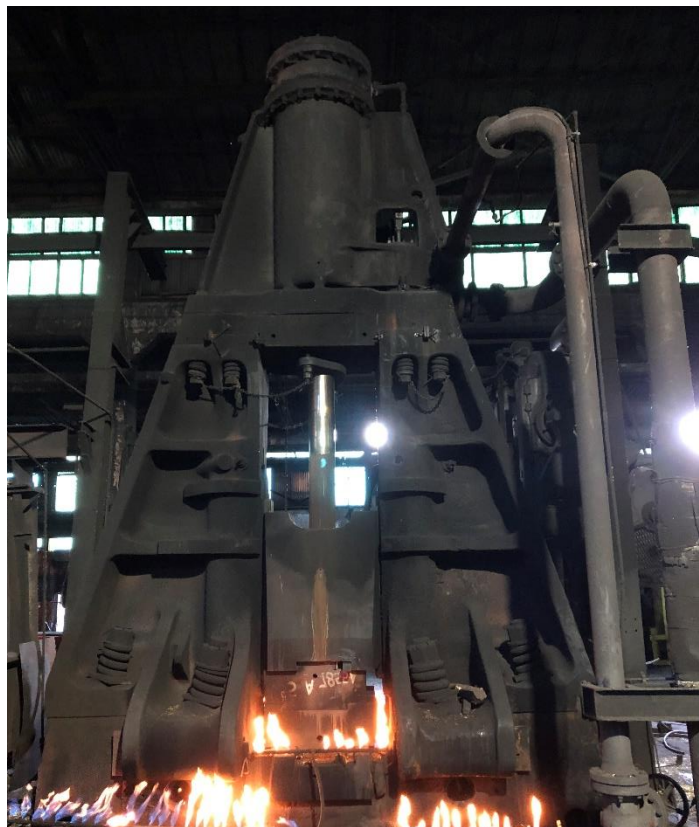
12,000# Chambersburg Power Forge Hammer
