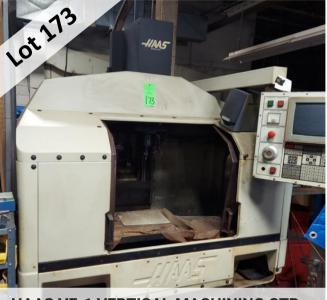
HAAS VF-1 VERTICAL MACHINING CTR.
