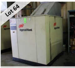
100HP ROTARY SCREW COMPRESSOR
